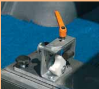
Locking latch for fixing the ramp inside.
