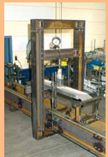
Altec loading ramps in manufacture. In the background is our automatic storage and selection system. Also shown is our capacity testing apparatus which is used as part of our in house quality control system.
